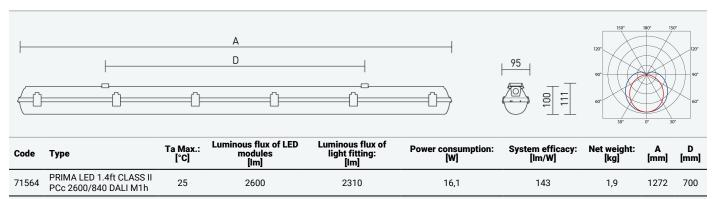
The values stated for power consumption and luminous flux are in a tolerance of  $\pm\,7.5~\%$
