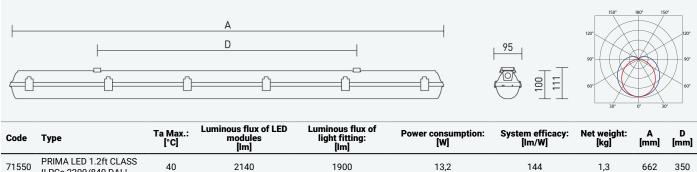
The values stated for power consumption and luminous flux are in a tolerance of ± 7.5 %
