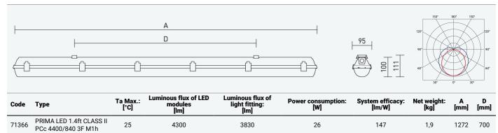
The values stated for power consumption and luminous flux are in a tolerance of  $\pm$  7.5 %
