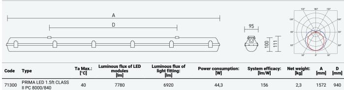
The values stated for power consumption and luminous flux are in a tolerance of  $\pm\,7.5\,\%$
